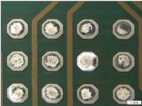
Fig. 7: 6 months storage + refresh + 3x reflow and wetting by wave soldering
