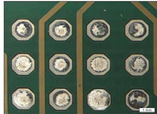
Fig. 8: 12 months storage + refresh + 3x reflow and wetting by wave soldering<sup>[FRH09]</sup>
