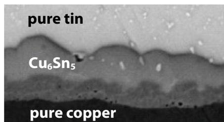
Fig. 2: Layer structure Cu/ Sn
