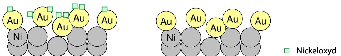
Fig. 11: Schematic description of the nickeloxide resolution<sup>[ATM11]</sup>
