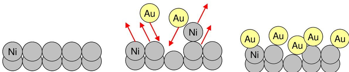
Fig. 9: Schematic description of the electroless Ni/ immersion Au process<sup>[ATM11]</sup>
