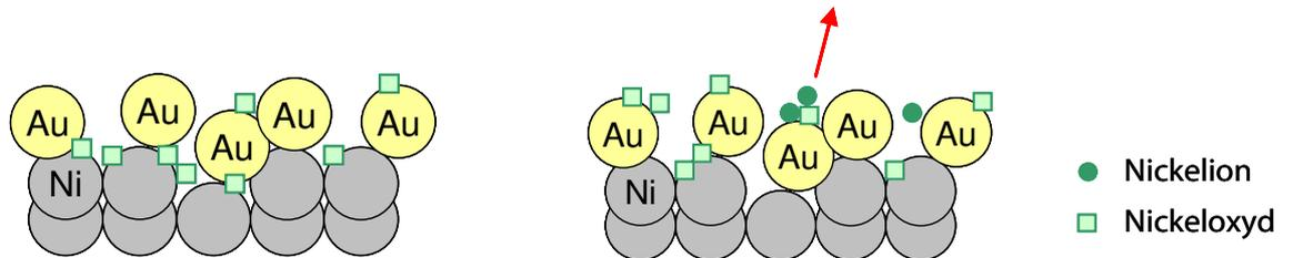
Fig. 10: Schematic description of the nickeloxide formation<sup>[ATM11]</sup>
