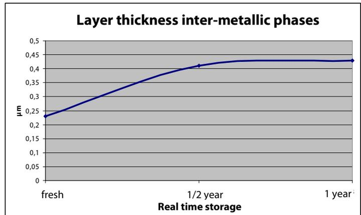
Fig. 3: Growth of inter-metallic phase/ real time storage<sup>8</sup>
