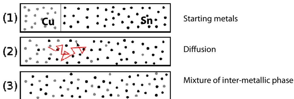
Fig. 1: Schematic representation of diffusion mixing<sup>1</sup>
